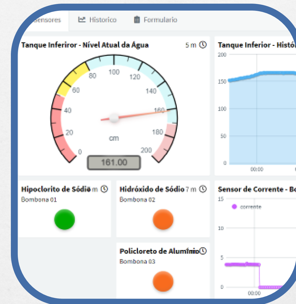
CENTRAL DE CONTROLE OPERACIONAL
